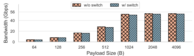
Figure 5: Bandwidth for different packet sizes with and without the switch.
