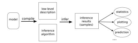
The ProPPA software framework contains a number of different inference engines, suitable for models with different characteristics, including infinite state space.
