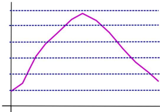
We can discretise the continuous range of possible concentration values into a number of distinct states. These form the possible states of the component representing the reagent.
