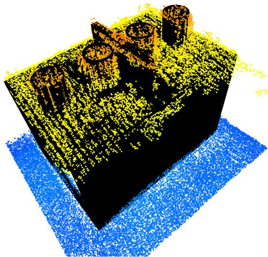
(a) Registered CAD model (black) after the two step registration procedure
