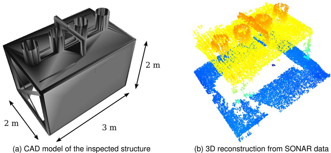
Fig. 1. 3D reconstruction of oil-field-type structure from multibeam SONAR observations.
