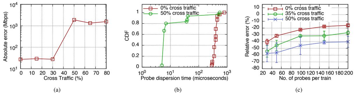
Fig. 8. (a) Accuracy of capacity estimation with WBest; (b) CDF of dispersion times from 30 probe pairs used for WBest’s capacity estimation phase; (c) Accuracy of WBest with known capacity for varying probe train sizes and cross-traffic levels. All cases correspond to Scenario 1 when FA is ON.
