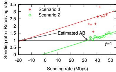
Fig. 6. Different estimation behaviors of DietTopp at 80% cross-traffic rate in Scenarios 2 and 3 when FA is ON.
