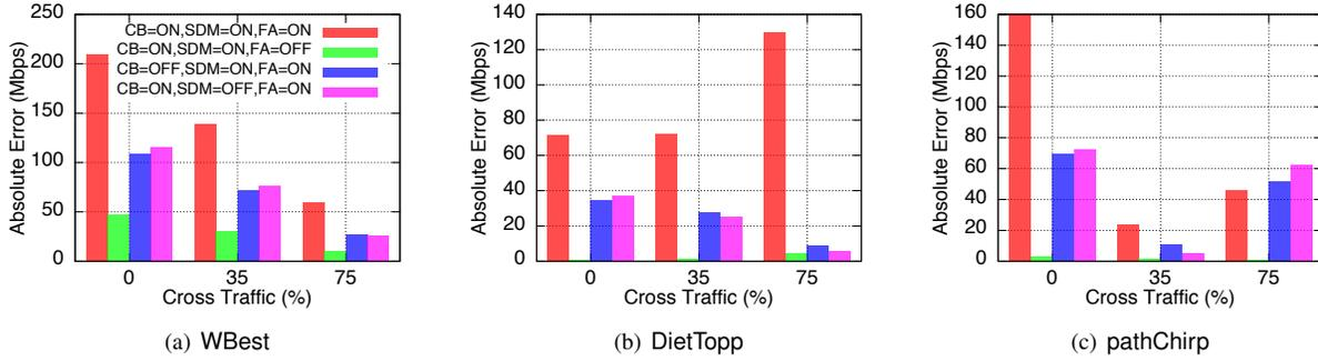
Fig. 2. Relative impact of key 802.11n features (FA, channel bonding (CB) and spatial division multiplexing (SDM)) on the accuracy of different ABE tools in Scenario 1 (see Figure 3).
