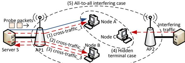
Fig. 3. Schematic of testbed and various cross-traffic scenarios.
