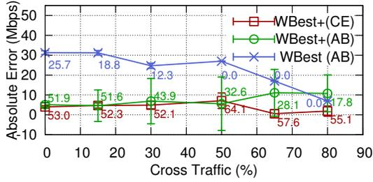
Fig. 9. Accuracy with WBest+ in Scenario 1 when FA=ON. Numbers next to data points denote actual estimation values.
