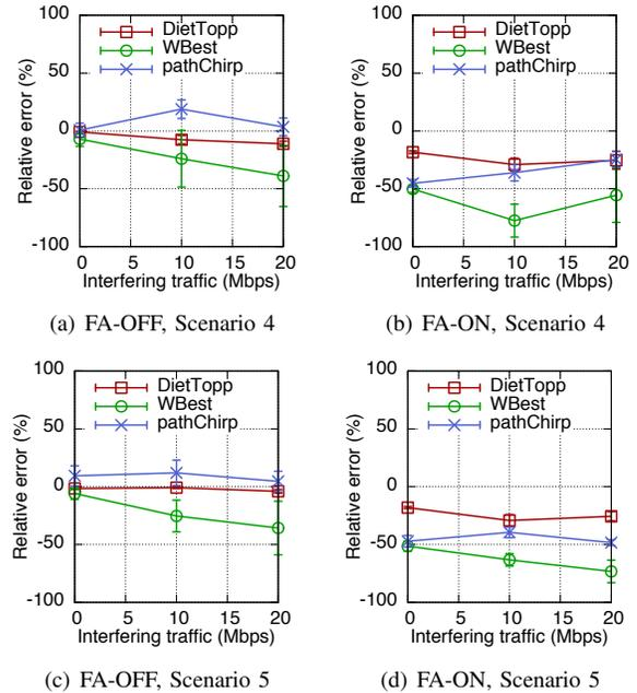
Fig. 7. Accuracy of the three tools in Scenarios 4 and 5. The median relative error across all cross-traffic levels for DietTopp, WBest and pathChirp are: 8%, 24% and 3% when FA is OFF in Scenario 4; 27%, 59% and 33% when FA is ON in Scenario 4; 2%, 25% and 9% when FA is OFF in Scenario 5; 26%, 63% and 47% when FA is ON in Scenario 5.
