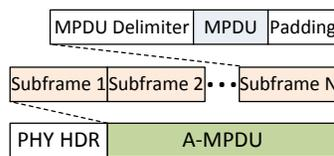
Fig. 1. A-MPDU type frame aggregation.
