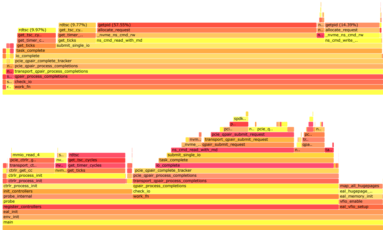
Figure 6: Flame Graphs for Intel SPDK running inside Intel SGX enclave plotted using TEE-PERF: (top) unoptimized version of SPDK, and (bottom) optimized version of SPDK.
