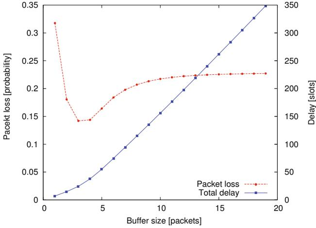
**Fig. 6.** Packet loss & delay behaviour as buffer size is varied. ALOHA network ( $n = 10$ ).
