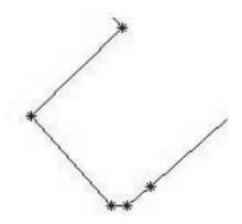
Exploit problem constraints: long lines, meet at given angles — delete short badly placed segments and extend to intersection
