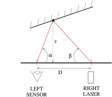
you can see how the ray at angle  $\beta$  from the laser intersects the viewpoint at angle  $\alpha$  from the sensor. If you know the distance D between the two then simple geometry can be used to calculate the distance z.
