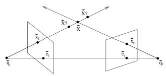
Estimate ?  $|\vec{e}_l, \vec{e}_r|$ , by exploiting  $\vec{e}_r$  ' $F = F\vec{e}_l = \vec{0}$
