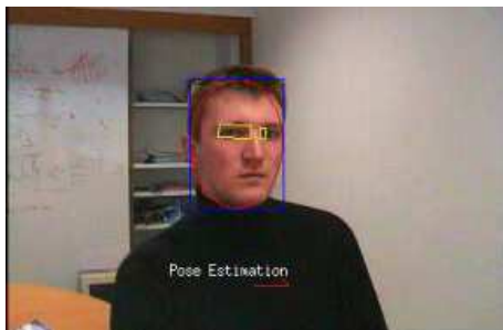
Figure 12. Real-time head pose estimation.
