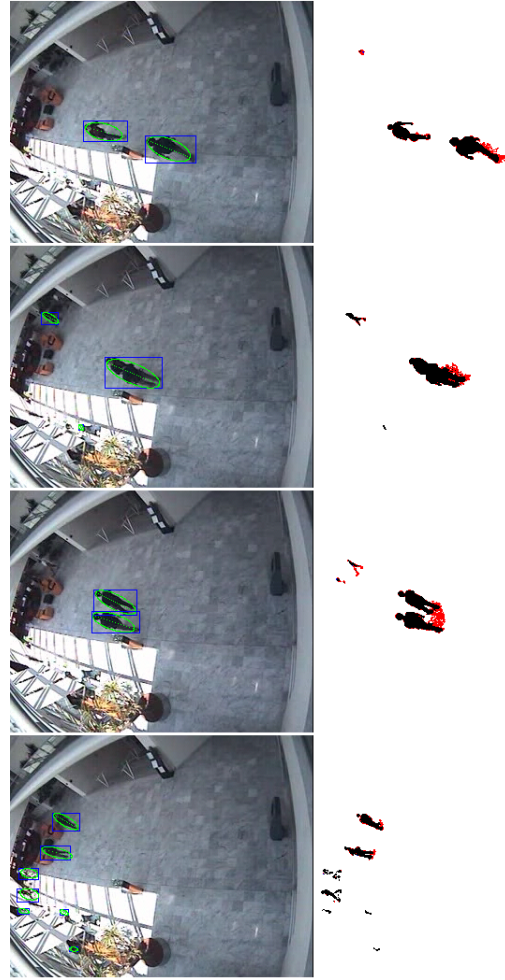
Figure 5. Pedestrians detection using the PETS04 dataset
