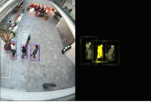
Figure 2. Target tracking by background differencing. The central person is tracked using all pixels whereas the two other persons are tracked using every second pixel.
