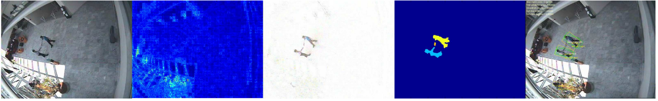
Figure 1: Tracking results (from left to right): Original frame; Model of the background variances; Results of background subtraction; Detected blobs after morphological operations; Resulting tracked objects (outlined in green) with ground truth data and results shown in yellow.
