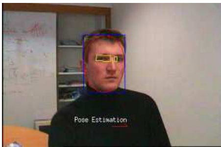
Figure 12. Real-time head pose estimation.
