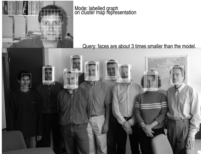
Fig. 7. Successful detection of faces in unconstrained images. The white rectangles mark the position and size of the graphs with lowest cost.
