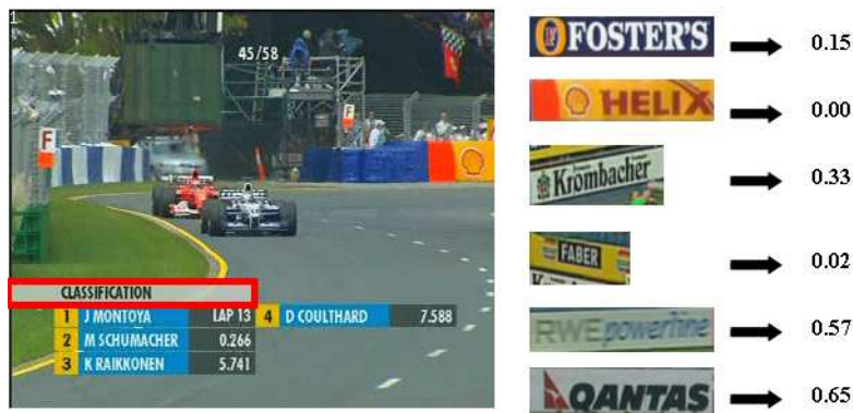
Fig. 6. Example of a difficult case. The module confuses the gray box marked classification with the qantas logo.
