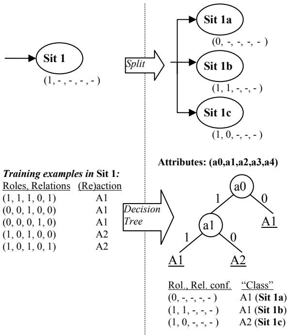
Figure 4: Splitting Situations with Decision Tree algorithm (ID3).
