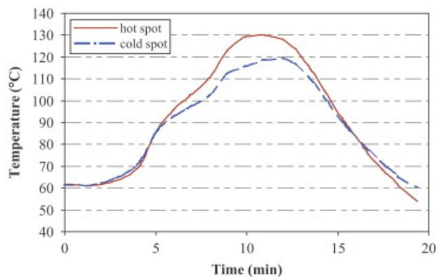
**Figure 4. Validation of cold and hot spots locations specified by computer vision method [1]**
