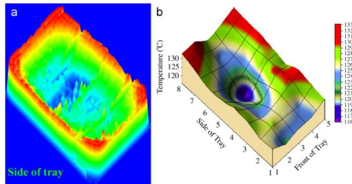
(a) Heating pattern by developed computer vision method.
