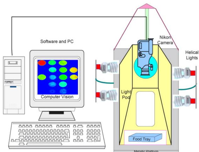
Figure 1. Computer Vision Hardware setup [1]
