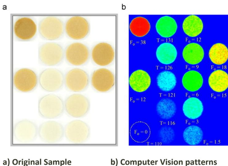
Figure. 3. Computer vision patterns for mashed potato samples heated to a set temperature of 121°C for different F0 (thermal lethality of target microorganisms) [1]
