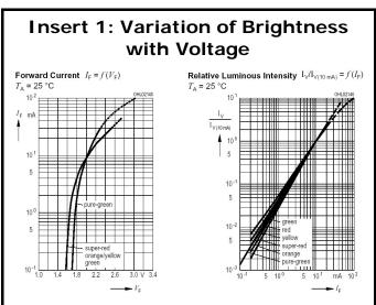
The right hand graph shows how light output varies with current, for the LS -3340 range from Osram. The response is nearly linear and the output can be easily controlled using currents from 0.2mA to 20mA.
