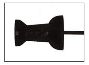
Even when an object is transparent, the resulting image appears as a black silhouette because of the collimated illumination. This occurs when the collimated light passes through the transparent resin and is refracted, so that the light does not pass into the camera. This technique can be used to accurately check the dimensions of transparent objects.
