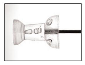
If diffused light is used as backlight, as is the case above, the light can pass through the transparent object making any internal air bubbles or embedded metal parts clearly visible. These imperfections can then be easily recognised. This technique can be used to check on the quality of the moulding process.
