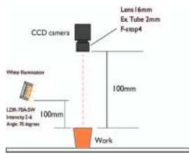
The lighting setup is shown next to the image. The illuminator uses white light with the result that both the printed date *and* the picture of fruit are evenly illuminated. This makes the job of OCR much more difficult as the software has a much harder job separating out the text from the background.
