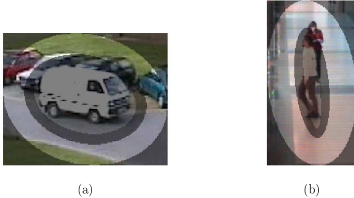
Figure 5: Examples of a centre-surround model with safety margin. (a) Tracked van from a traffic-monitoring sequence. (b) Tracked person from an indoor surveillance application in a shopping centre. Regions from centre to border: target estimation, safety margin, surrounding background, and non-local background.
