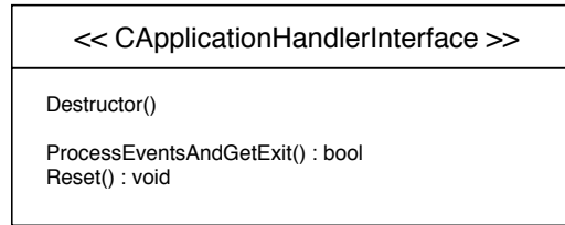
Fig. 2.3. Representation of the methods of the interface CApplicationHandlerInterface in UML.
