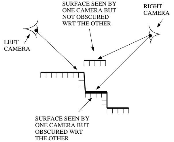
Figure 8: Geometry of the consistent surface constraint geometry.
