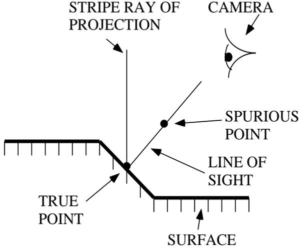
Figure 6: Geometry of the illumination direction constraint.
