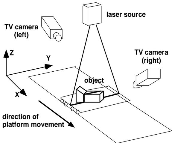
Figure 2: Architecture of the range sensor.
