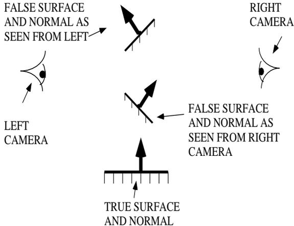
Figure 9: Geometry of the unobscured-once-viewed constraint.
