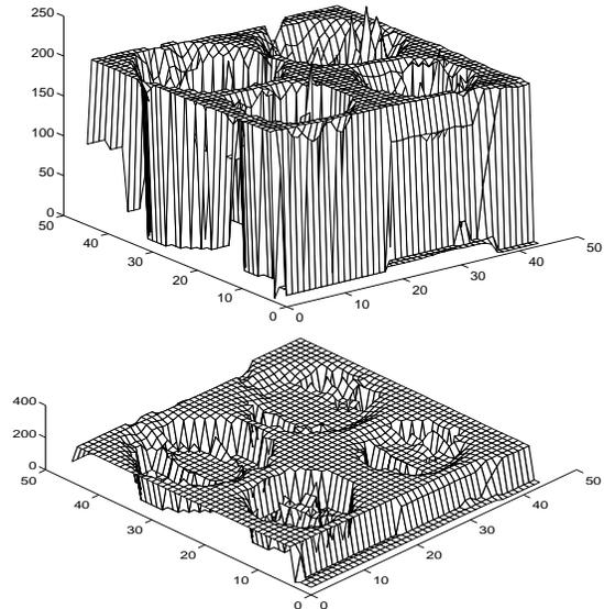
Figure 10: Range image of block with holes with consistency tests enforced.
