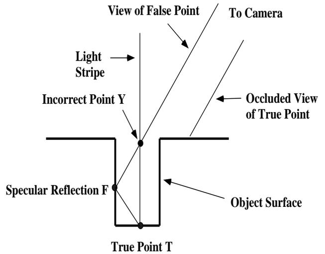
Figure 5: How specular reflections cause false range values.
