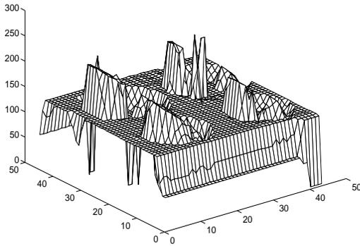
Figure 1: Two range images of polished aluminium block with holes. Specular reflections make spurious surfaces appear.
