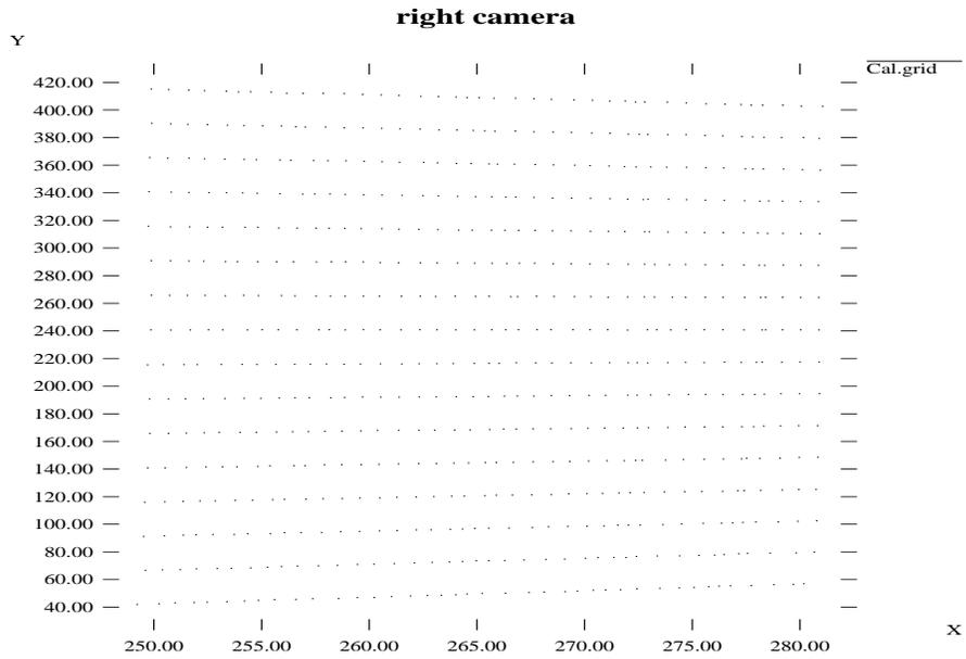
Figure 4: Calibration grid for 80 height levels (steps).
