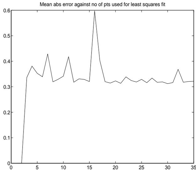
Figure 6: Mean absolute error of least squares plane fit against number of points used.
