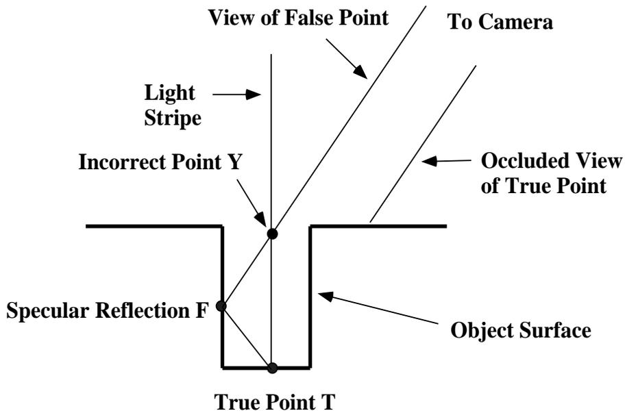
Figure 5: How specular reflections cause false range values.
