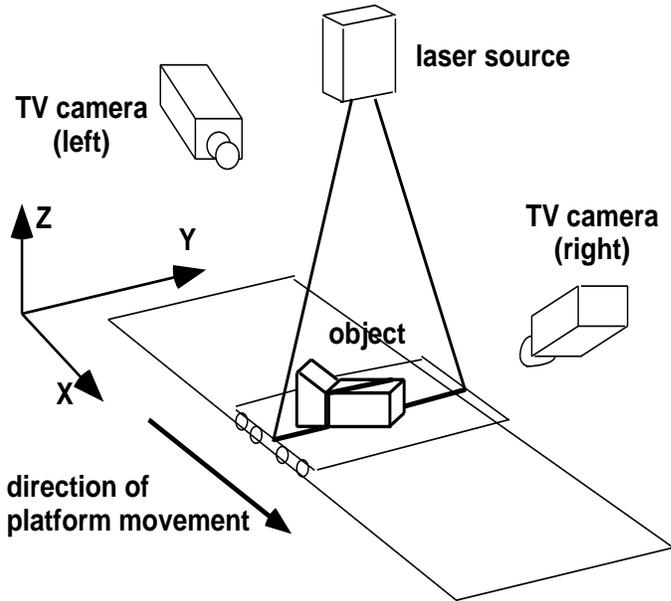
Figure 2: Architecture of the range sensor.
