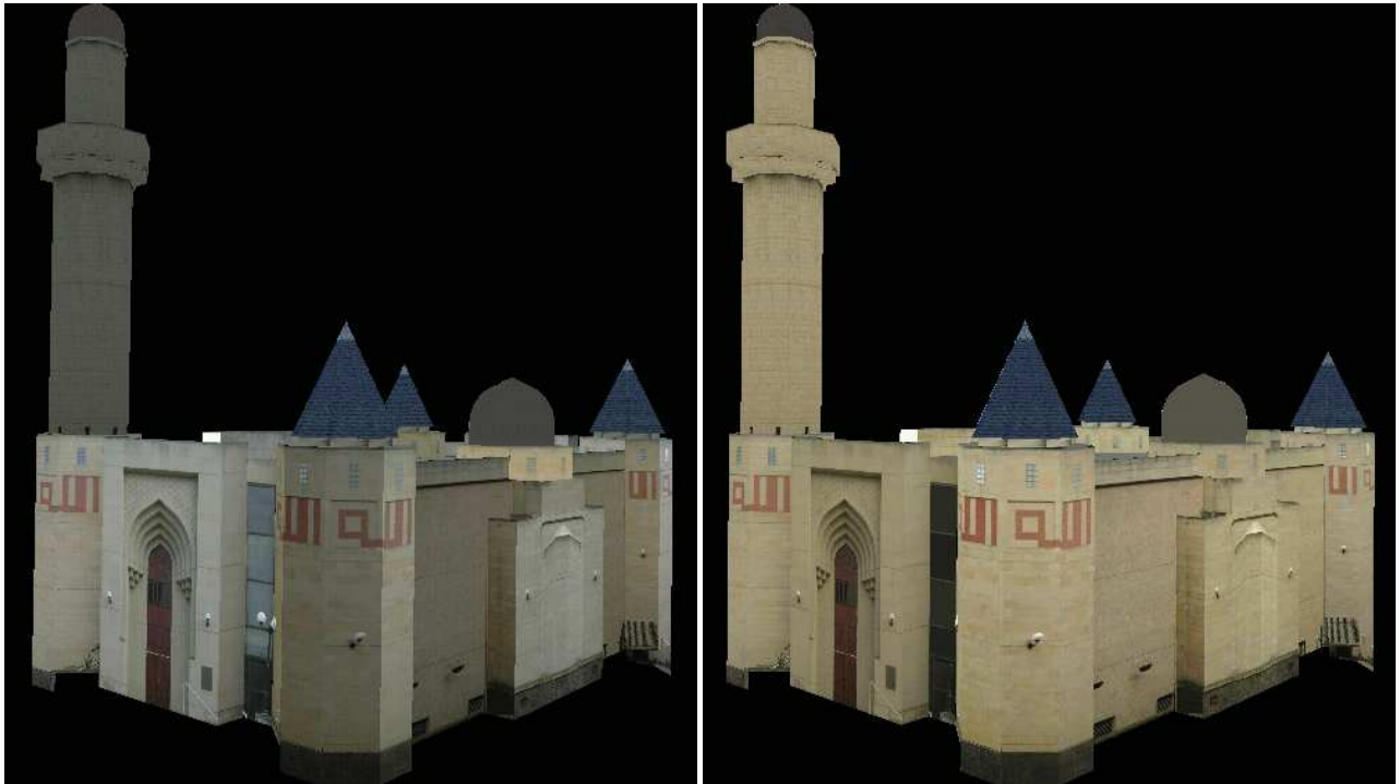
Figure 8. A VRML model textured with 30 original images (left) and color corrected images (right). The color correction method was applied several times. The appearance of all stone surfaces is much more consistent than the original.
