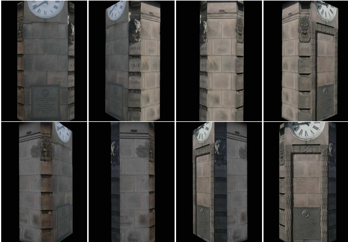
Figure 9. A VRML model textured with eight real images before the color correction. Image 1 is the top leftmost image. The image numbering starts from the top leftmost in a clockwise direction. There are some color discrepancies at image boundaries.
