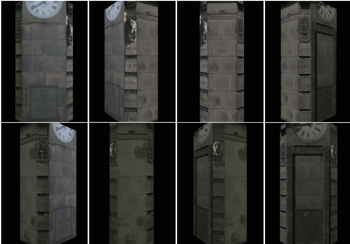
Figure 11. A VRML model textured with eight real images after the pairwise color correction. Image 1 is the top leftmost image. The image numbering starts from the top leftmost in a clockwise direction. Color discrepancies at image boundaries were almost removed. However, there is a large dissimilarity between the front face of the tower and overlapping region 4 due to the error accumulation.
