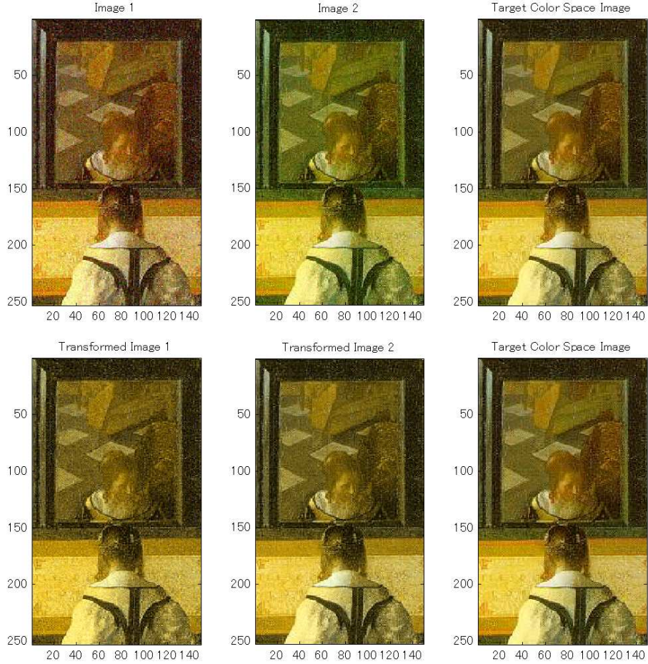
Figure 5. The top row images show test set, image 1 (left), 2 (middle) and a target color space image (right), in the overlapping region before the color correction. The bottom row shows the result images after the color correction. Gaussian noise is added to the reference color space images.
