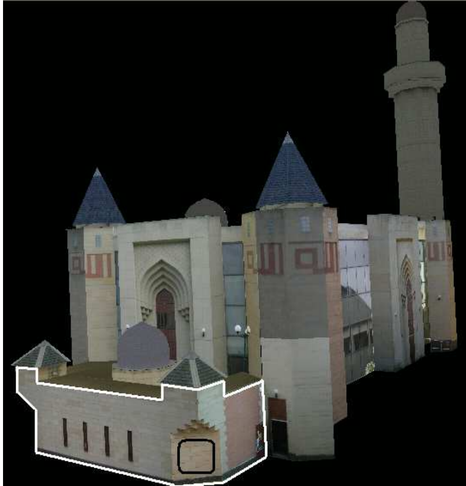
Figure 1. A VRML model texture mapped using 30 images. The highlighted line region consists of three different images seen from right, bottom and left directions. The dark oval surrounds the overlapping region. The model has color discrepancies at the image boundaries.
