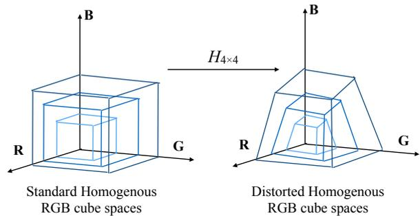
Figure 2: Homogeneous color space mapping. The left 3 homogeneous RGB cubes are equivalent (up to a scale). The left RGB space cubes can be mapped to the right by a  $4 \times 4$  3D homography transform  $H$ .
