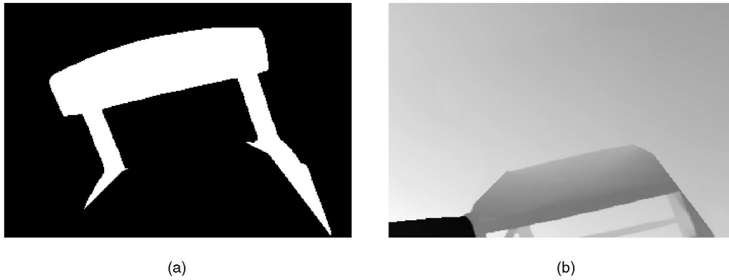
Fig. 5. (a) Map of occluded lines, in white in a black background. (b) Range image after occluding points have been replaced by estimated occluded points (compare with Fig. 1a).
