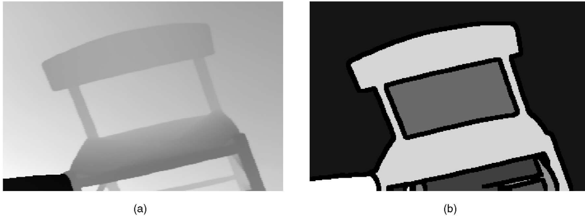
Fig. 1. (a) A range image and (b) corresponding extracted regions after labeling.
