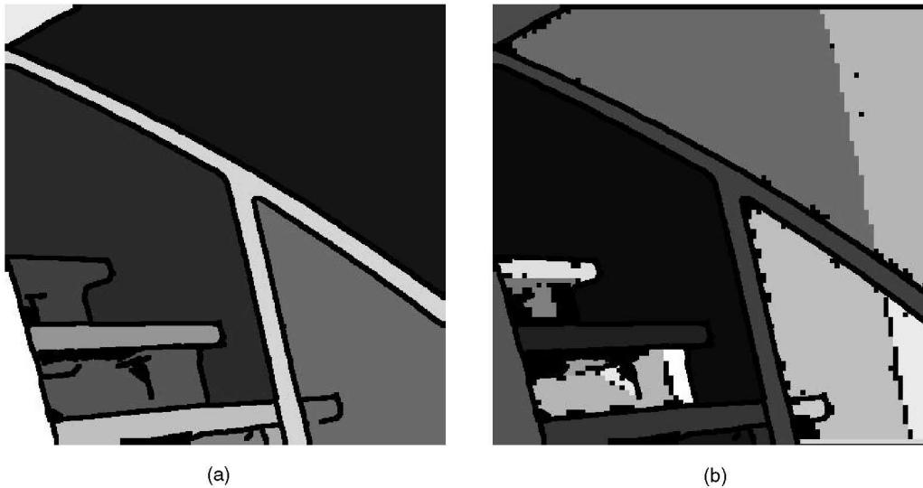
Fig. 3. The image in Fig. 2 after some processing. (a) Partitioned using only depth discontinuities. (b) Additionally partitioned using also fold edges.
