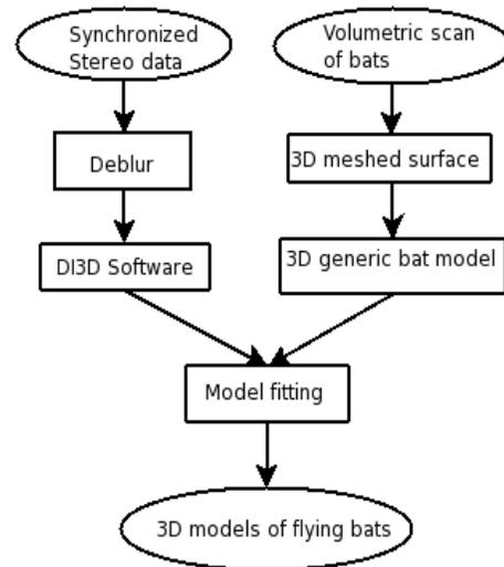
Figure 7 Diagram of recovering 3D bat shapes
