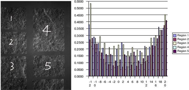
Fig. 2. (a) test plane; (b) RMS error (mm) for regions in (a)
