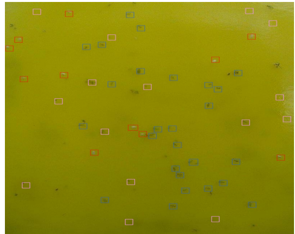
Figure 5: Classified regions with red blobs for whitefly and pink for background (no fly regions) and blue are for greenfly. Insect count is displayed to the user. All whiteflies are classified correctly while we have 4 false positives w.r.t greenfly count. This is since there are some rare insect which has same shape as greenfly and are of black color.
