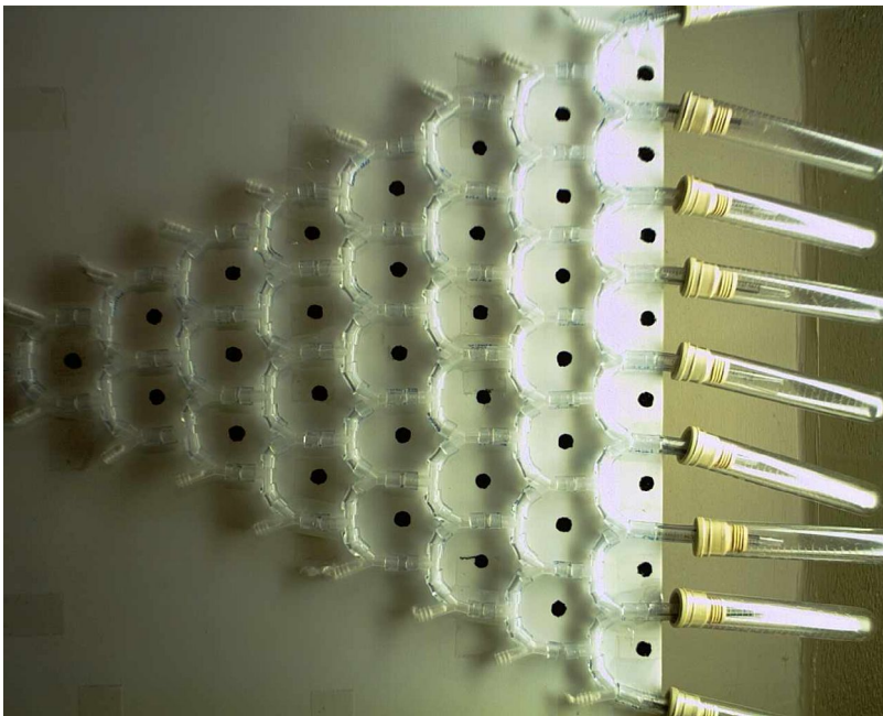
Figure 2.2.1: The gravity maze, viewed from the recording camera (though the video footage is not in colour). Flies enter at the the left and progress to the test tubes on the right, attracted by a light gradient (which can be seen in the picture). Exits are numbered 1 (bottom) through 9 (top). Note that the T-junctions appear in 8 columns, which we shall refer to as column 1 (left, consisting of just one junction) through column 8 (right).
