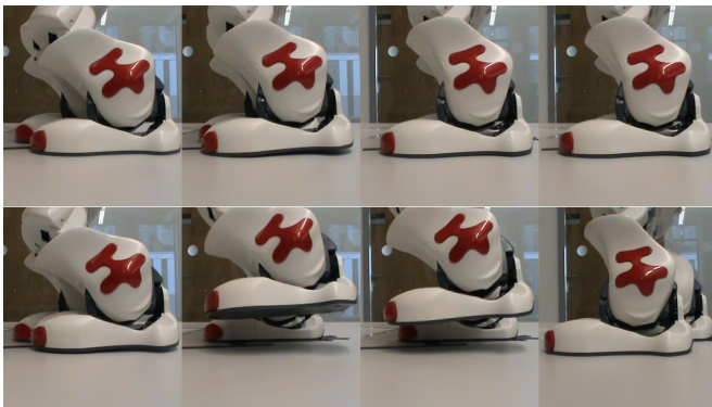
Fig. 24. Detail of a left foot swing. Top ; the original trajectory that provides minimal foot clearance (approx. 2cm on apex). Bottom ; adding a obstacle close to the original trajectory pushes the optimization to higher stepping trajectories (here approx. 5cm on apex).
