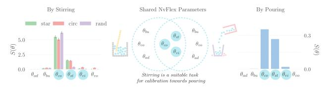
Fig. 4. Model sensitivity analysis for six NvFlex parameters affecting liquid behaviour in simulation for (Left) Stirring using different patterns (star, circular, and random) and (Right) Pouring. We are interested in the shared parameter between tasks (Middle). Parameter names are abbreviated as (ad: Adhesion, bu: Buoyancy, co: Cohesion, st: Surface Tension, vi: Viscosity, vo: Vorticity).
