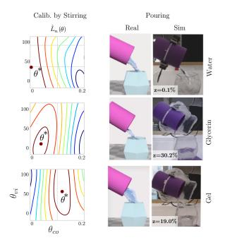
Fig. 8. (Left) Contour plots of the likelihood of the fluid parameters after stirring water, glycerin and gel for one of the repetitions. (Middle) Pouring with the real robot. (Right) Synchronized pouring in simulation.
