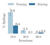
Fig. 6. Effect of two calibration methods in the deployment task measured as the decrease of spillage with respect to the number of iterations.
