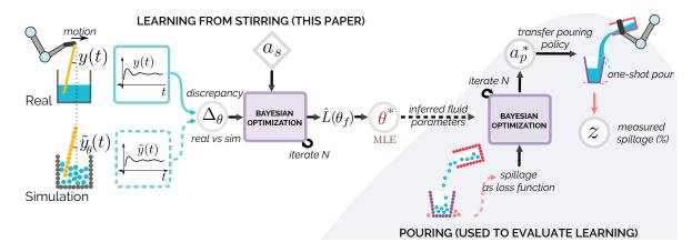
Fig. 2. This paper focuses on learning parameters of liquids by stirring. Learning parameters of liquids  $\theta$  by stirring with the motion pattern  $a_s$ . The discrepancy  $\Delta_{\theta}$  between the real y(t) and simulated  $\tilde{y}(t)$  time signals is obtained in real time. The efficacy of learning is evaluated by executing one-shot pouring and measuring the percentage spillage z.
