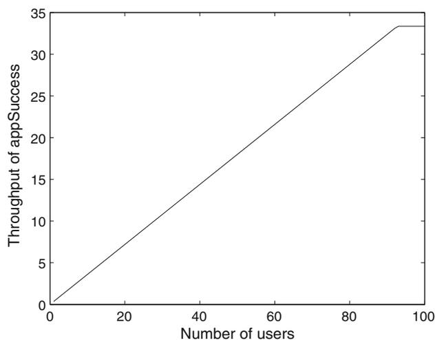
**Fig. 13** Workload analysis studies how the user population affects performance of the system. Here, the performance metric of interest is the steady-state throughput of processing applications to e-University courses. Non-degrading performance is observed for population sizes less than 93
