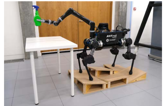
Quadruped robot equipped with an arm performing a task over uneven terrain.
