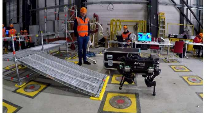
Fig. 1. ORCA project testing: a quadruped robot was teleoperated to traverse industrial scaffolding, and eventually pressed an E-stop button, while thermal information was fed-back to the operator.
