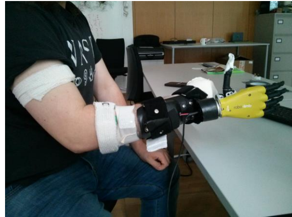
Fig. 3. Twelve electrodes were placed on the subject's forearm and securely fixed with an elastic bandage. The subject's fingers were constrained with bandage as well and the prosthetic forearm was mounted on the hand using a specially designed socket for this purpose.
