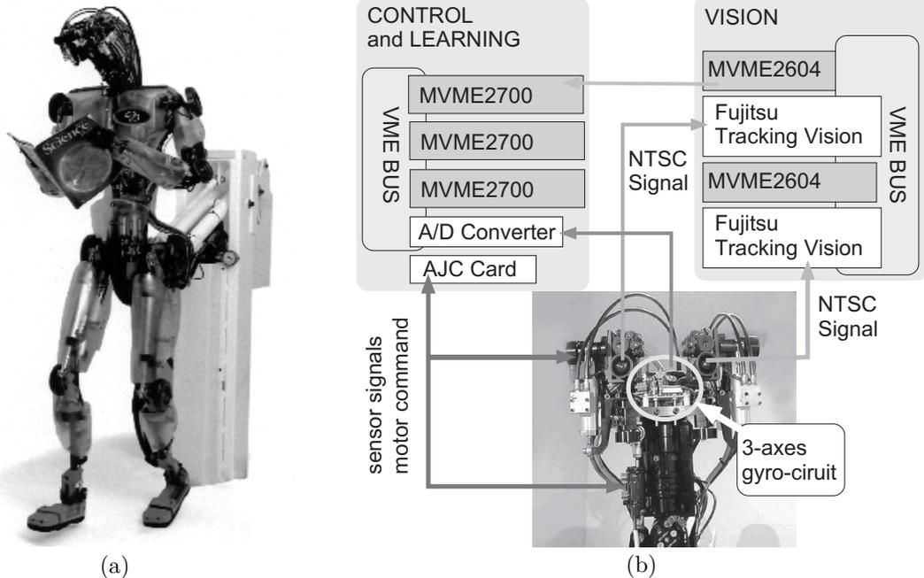
Figure 3: (a) The 30 DOF Humanoid robot used as a testbed for implementation (b) The experimental setup of the humanoid vision-head system
