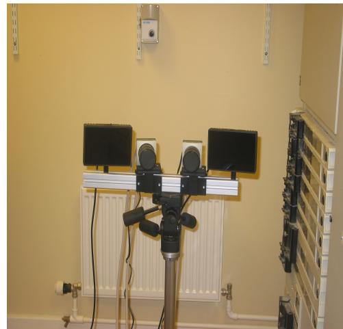
Fig. 1. Stereo rig of the high-speed scanner
