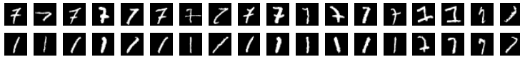
Figure 8: The Nearest Neighbour method makes 18 errors out of the 600 test examples. The 18 test examples that are incorrectly classified are plotted (above), along with their nearest neighbour in the training set (below).
