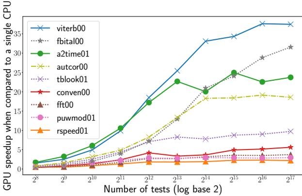
**Figure 5: Speedup on the GPU vs single thread execution for 10 different test suite sizes. GPU data transfer and kernel execution not overlapped.**
