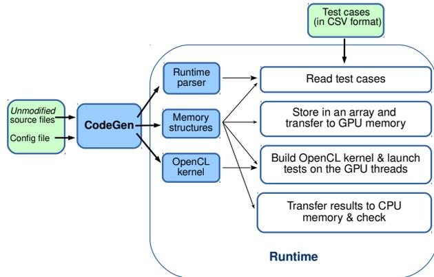
Figure 1: ParTeCL: automated test execution on the GPU.
