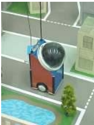
Figure 2: The robot is built on a 8cm x 8cm base. Its wireless color video camera sends images to a PC for processing, and the PC send motion commands by radio to the robot.
