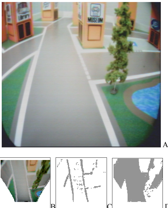
Figure 3. B: Top view obtained from a perspective transform of A. C: Extracted road edges. D: Extracted road surface areas.
