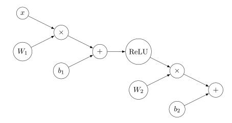
The graph is called a computation graph, where every vertex is either a variable or an operation. When values are given to the variables, we can run the computation graph to get the result of the computation. We hope to write the following snippet that prints the value of the output.
