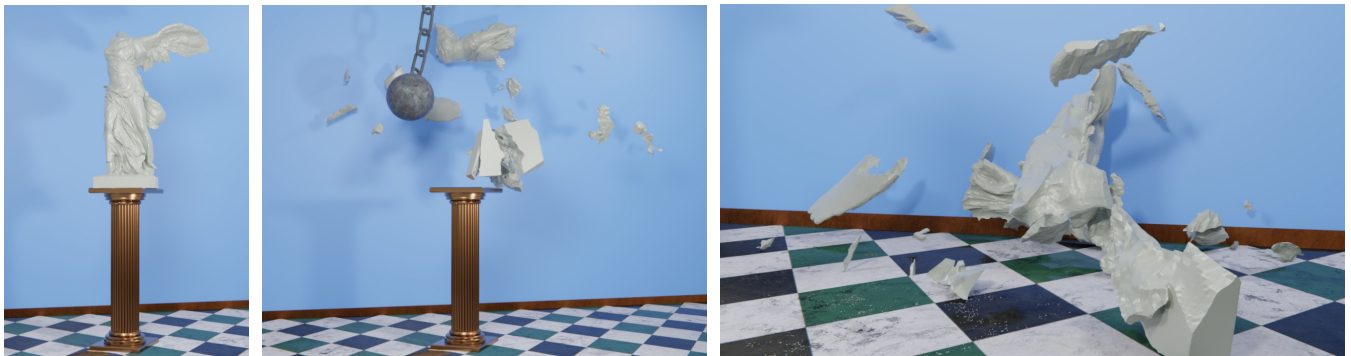
Figure 1: Our method offers a high-resolution crack propagation scheme on an explicit surface mesh without the need for adaptively tetrahedralized input meshes. We achieve this by combining a novel adaptation of the extended finite element method (XFEM), and a polygon-based cutting algorithm to compute fragments which retain their characteristic ridge-like structures—and sharpness—due to cracks. The figure shows an impact between a statue of The Winged Victory of Samothrace and a wrecking ball.
