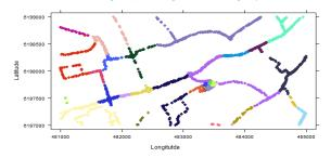
Fig. 5: Final irregular tessellation (reflecting the basis of ZipWeave non-uniform sampling) on routes (after applying Constrained Clustering + DBSCAN, we obtain 38 route segments).
