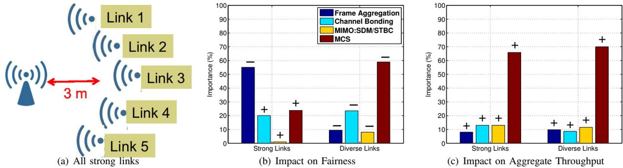
Fig. 10: Relative impact of 802.11n features on fairness and aggregate throughput performance in different network scenarios.
