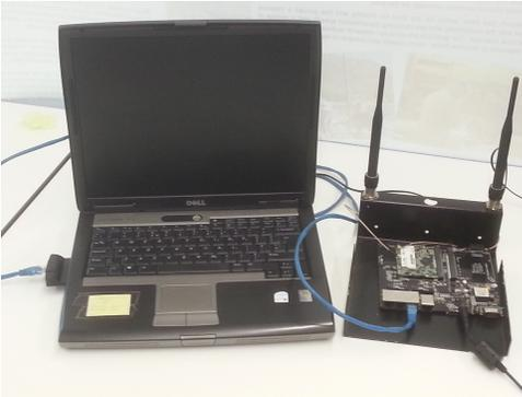
Fig. 2: Picture of a node in our 802.11n WLAN testbed.
