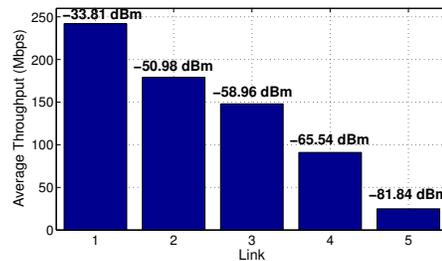
Fig. 3: RSSI and throughput variation across links in the testbed for a specific setting of values for 802.11n features.
