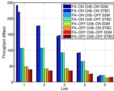
Fig. 5: Impact of frame aggregation, channel bonding and STBC/SDM on throughput with the default rate adaptation algorithm in use.
