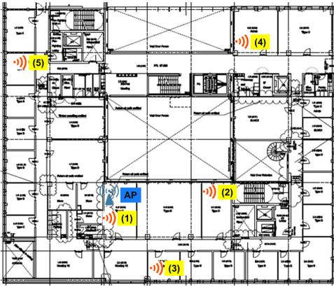
Fig. 1: Physical layout of nodes in the 802.11n WLAN testbed — the blue coloured node is the AP and red ones numbered (1)-(5) are stations.
