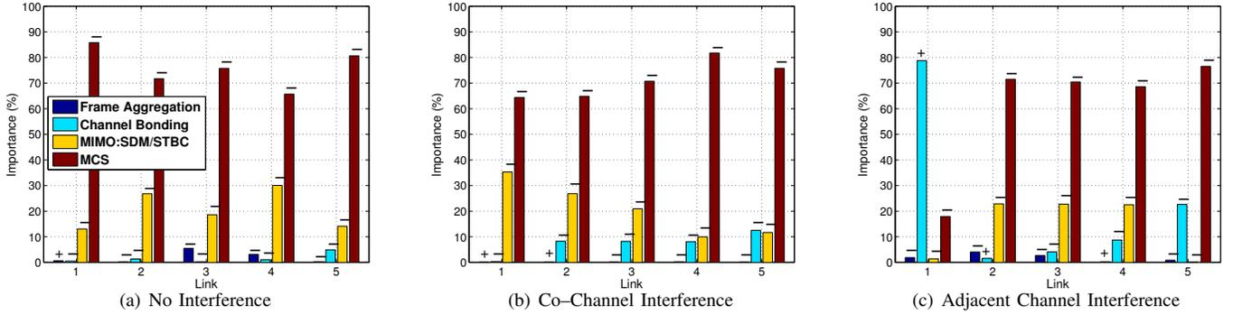
Fig. 7: Relative impact of 802.11n features on packet loss performance in terms of Pratt’s importance measure (section II.D) in different scenarios (channel quality and interference conditions).
