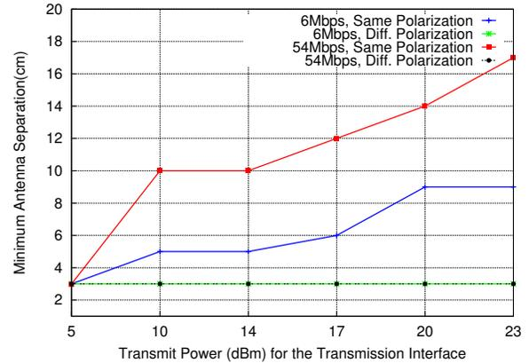
Fig. 3. Minimum antenna separation required to avoid throughput degradation on Avila based dual-radio 802.11 platform at different bit-rates, antenna polarizations and collocated interferer transmit power levels.
