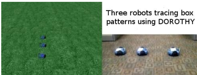
Figure 5: Three fluke robots drawing a box in synchronization with their virtual representations.
