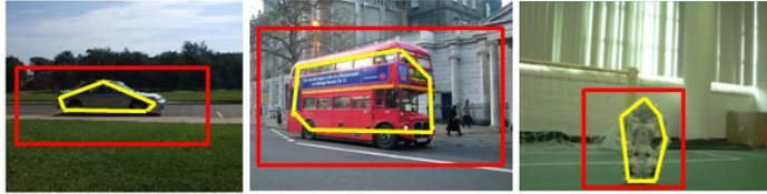
**Fig. 1.** Local, global and temporal cues extracted from pixels within the yellow boundary represent appearance, while mixture models and relative positions (e.g., “on” and “under”) of regions within the red rectangle (outside the yellow polygon) represent context.
