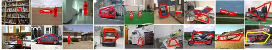
**Fig. 4.** Robot recognizes objects from different categories, multiple objects and multiple instances of an object in cluttered backgrounds. Last column shows an incorrect envelope (top) and an incorrect classification due to occlusion (bottom).
