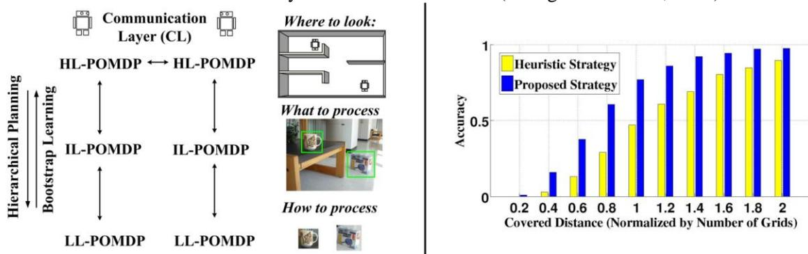
Figure 4: (Left) Layered POMDP hierarchy for visual sensing and information processing on a team of robots; (Right) Visual search based on constrained convolutional policies is more efficient than ad-hoc heuristic search strategies.
