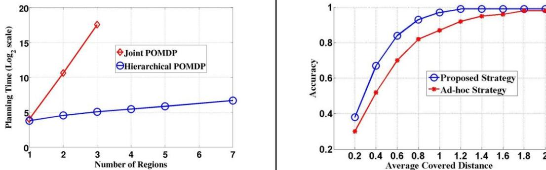
Figure 5: (Left) Hierarchical POMDP significantly reduces planning time in comparison to the POMDP over the joint state space of all image ROIs; (Right) Merging beliefs obtained by processing sensory cues with the communicated beliefs enables a team of robots to localize targets accurately while traveling a much smaller distance than with an ad-hoc probabilistic collaboration strategy.
