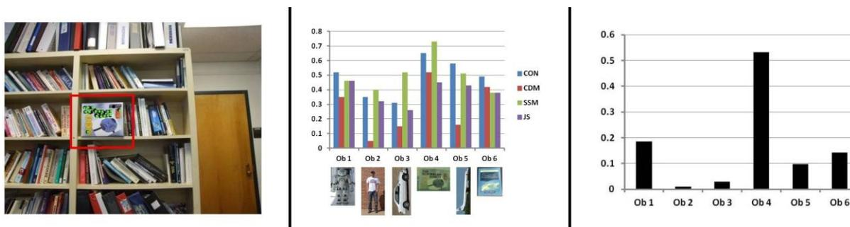
Figure 3: (Left) Test image of a box in a complex background; (Center) Individual match probabilities—the best subcategories within each category are shown along the x-axis; and (Right) Net match probabilities across different object categories—merging evidence from different components of the learned object models results in robust object recognition .
