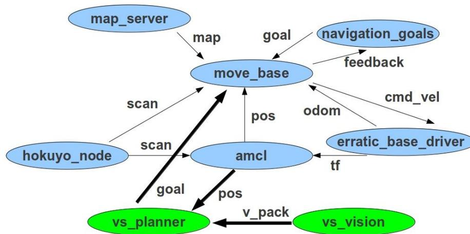
Figure 8: A ROS-based framework for integrating different components. Interaction between hierarchical planning, visual bootstrap learning and other control modules is illustrated.
