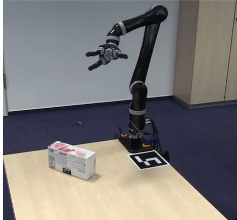
Fig. 5.13 The work done has been validated using a Kinova arm equipped with a Gripper KG-3. The goal was to grasp objects on a table using the framework developed in this chapter.
