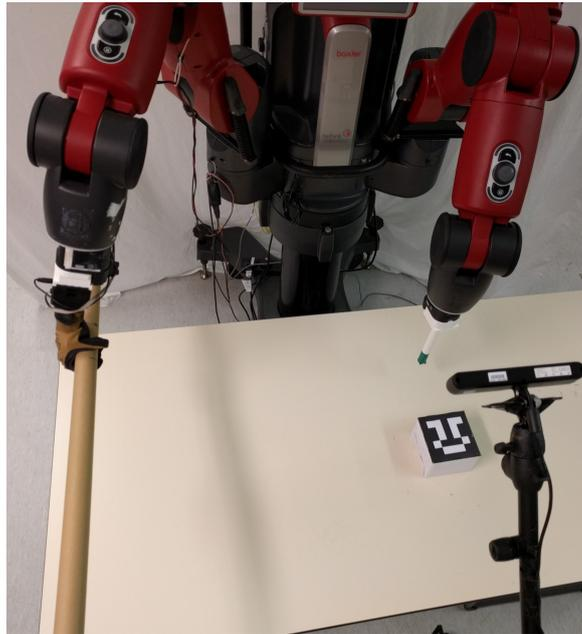
Fig. 1.4 The contributed uncertainty-calibrated model and model-predictive path integral control approach for pushing has been developed and evaluated on a Baxter robot platform. It has been equipped with a custom poking end effector on its left arm. The setup also includes an external RGBD sensor (Primesense Carmine 1.09) for object tracking.
