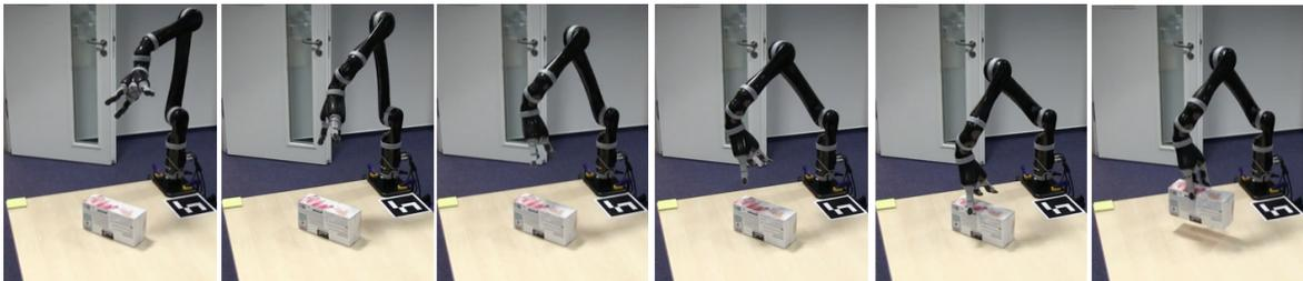
Fig. 5.14 Deployment of the approach on a Kinova platform equipped with a three-finger KG-3 gripper.
