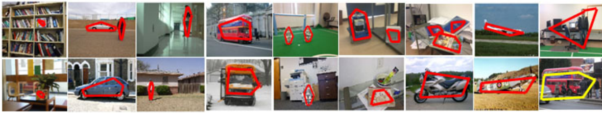
Fig. 3. Robot recognizes objects from different categories, multiple objects and multiple instances of an object in cluttered backgrounds. Last column shows an incorrect envelope (top) and an incorrect classification due to occlusion (bottom).
